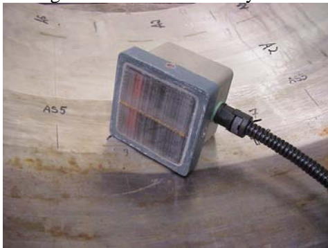
Probe Type: TS55 1.5. 6C1, 2x(2x16) elements, Angle 30 to 90°, foot print 54x54 mm
